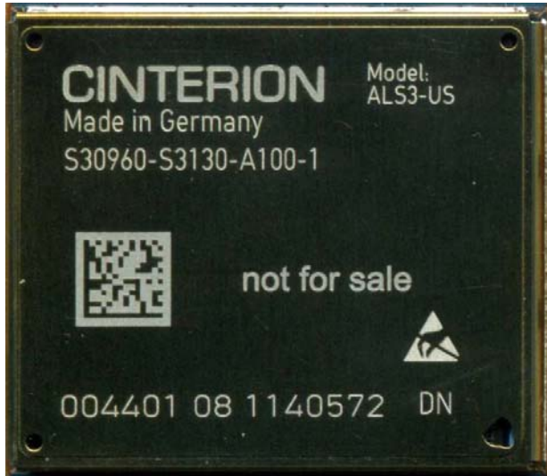
ALS3-US label location lasing on shielding
