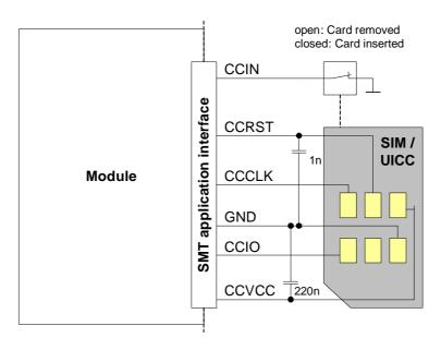
Figure 6: First UICC/SIM/USIM interface
