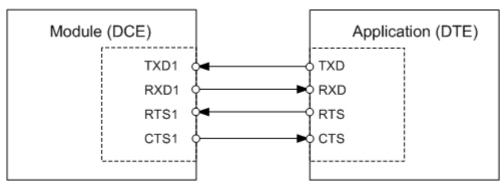
Figure 4: Serial interface ASC1
