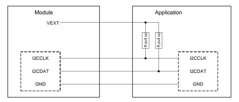
**Figure 5:** I<sup>2</sup>C interface connected to VEXT
