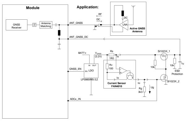
Figure 11: Supply voltage for active GNSS antenna
