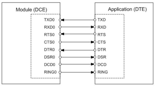
Figure 3: Serial interface ASC0
