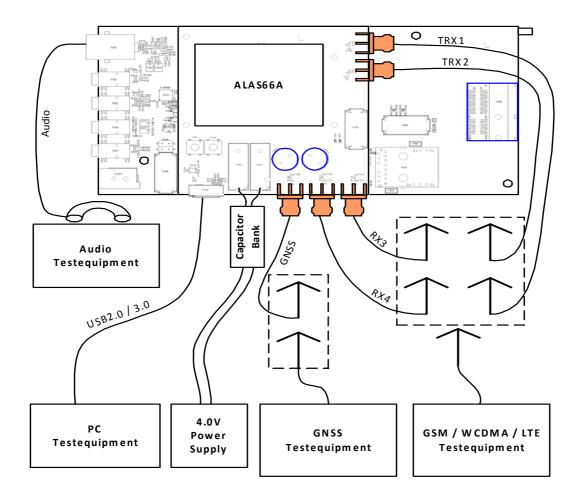
Figure 16: Reference equipment for type approval
