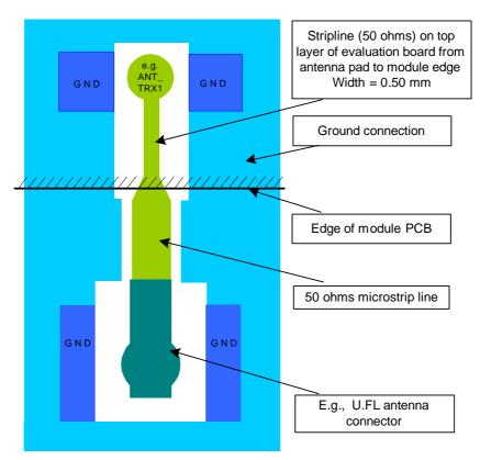
Figure 9: Routing to application's RF connector
