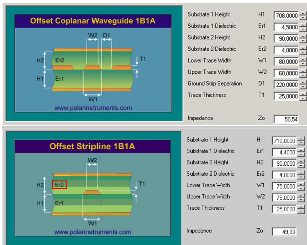
Figure 18: Embedded Stripline line arrangement
