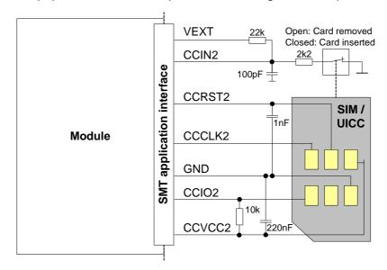
Figure 7: Second UICC/SIM/USIM interface
