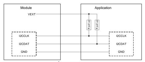
Figure 5: I<sup>2</sup>C interface connected to VEXT
