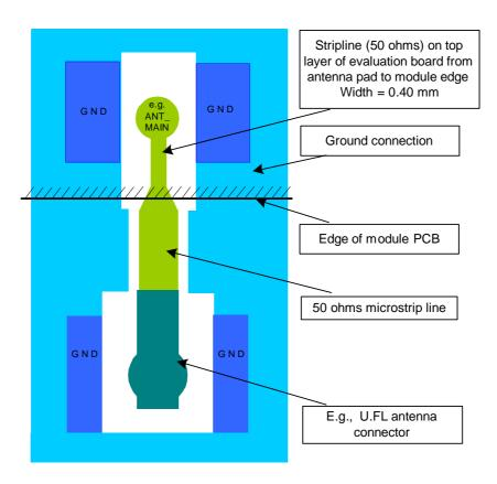
Figure 10: Routing to application's RF connector
