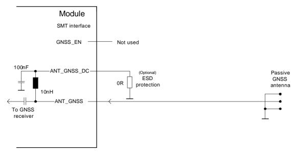
Figure 12: ESD protection for passive GNSS antenna
