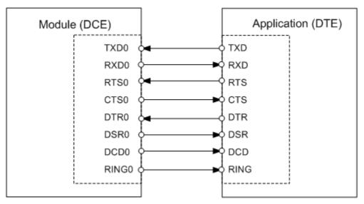
Figure 3: Serial interface ASC0
