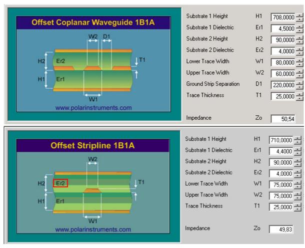
Figure 8: Embedded Stripline line arrangement
