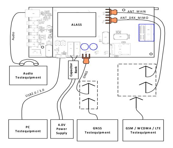
Figure 16: Reference equipment for type approval
