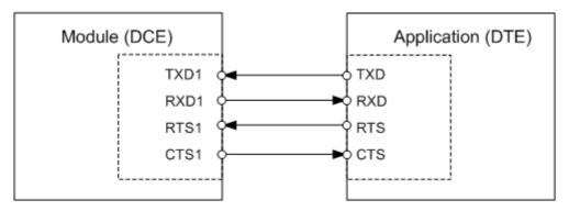
Figure 4: Serial interface ASC1
