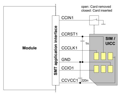
Figure 6: First UICC/SIM/USIM interface
