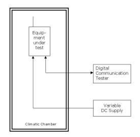
Principle set-up for tests under extreme test conditions
