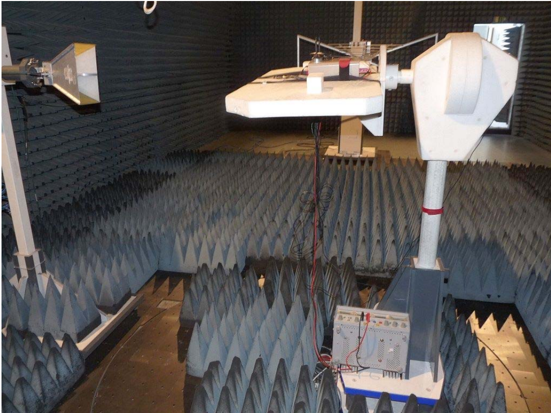
Photo 1: Test setup for radiated measurements (Enclosure, fully-anechoic chamber, 30 MHz – 10/20 GHz §22/24)
