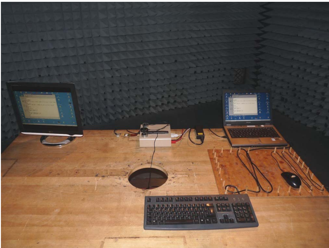
Photo 3: Test setup for radiated measurements (computer peripheral setup, EUT supplied by Serial-cable from computer, unintentional radiator $15)
