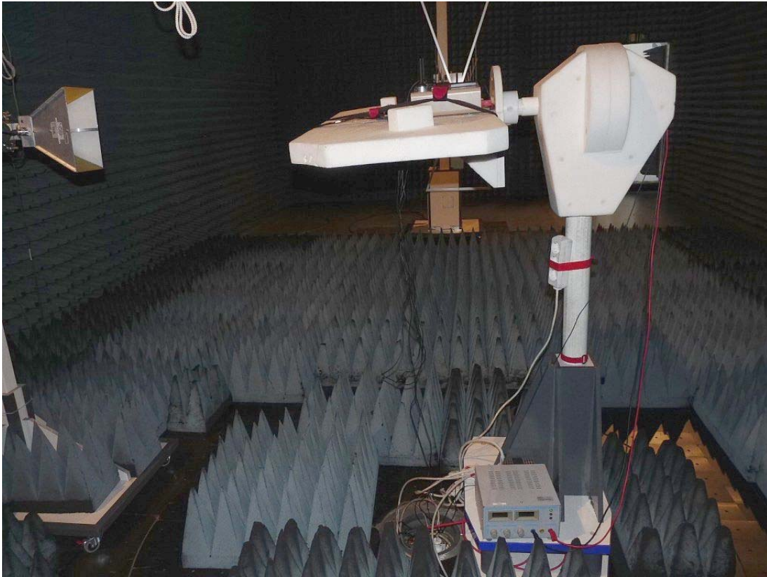
Photo 1: Test setup for radiated measurements (Enclosure, fully-anechoic chamber, 30 MHz – 10/20 GHz §22/24/27)
