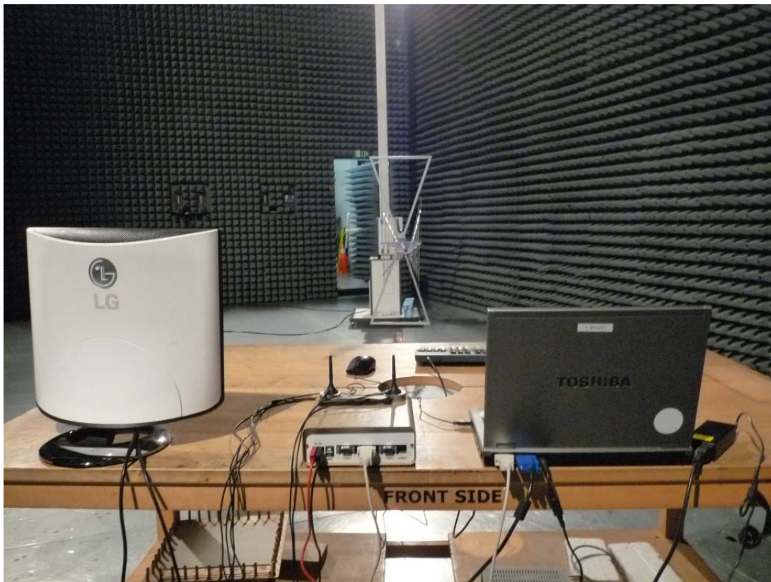
Photo 4: Test setup for radiated measurements (computer peripheral setup, EUT supplied by Serial-cable from computer, unintentional radiator $15)
