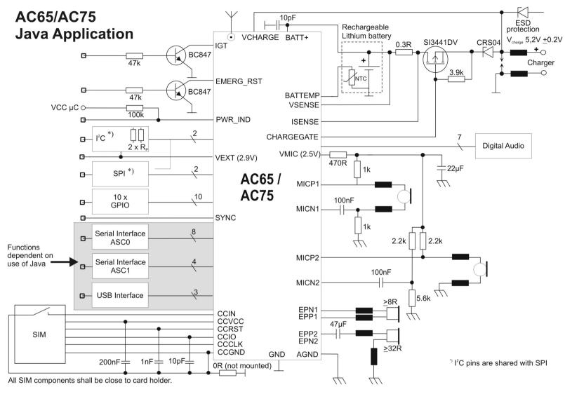
Figure 46: AC65/AC75 sample application for Java
