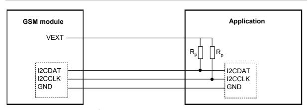
Figure 20: I<sup>2</sup>C interface connected to VEXT line of AC65/AC75
