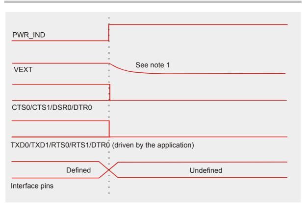
Figure 8: Signal states during turn-off procedure
