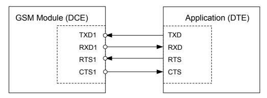
Figure 17: Serial interface ASC1
