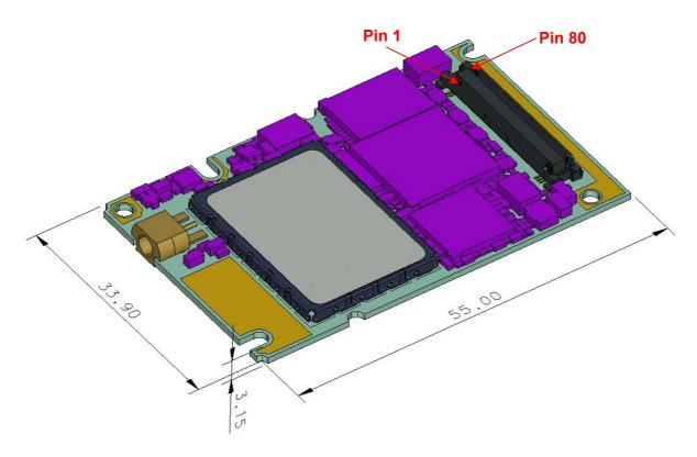
Figure 42: AC65/AC75 - top view
