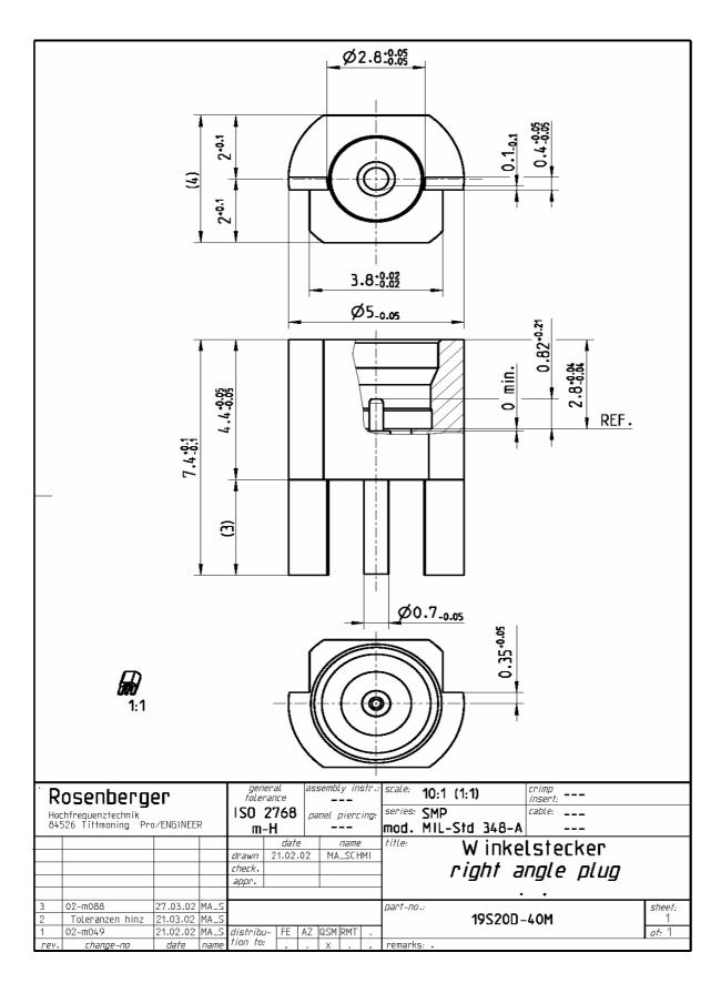
Figure 39: Datasheet of Rosenberger SMP MIL-Std 348-A connector
