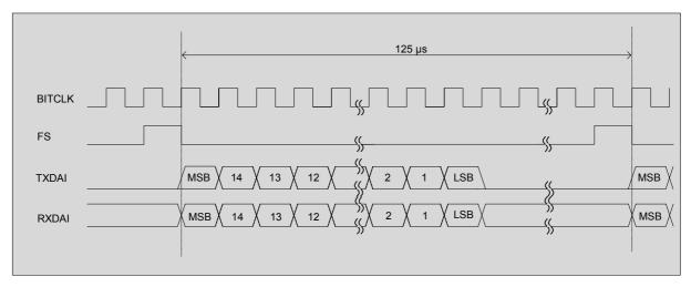
Figure 29: Master PCM timing, short frame selected
