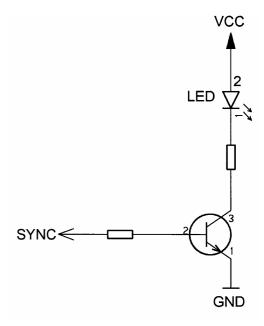
Figure 35: LED Circuit (Example)
