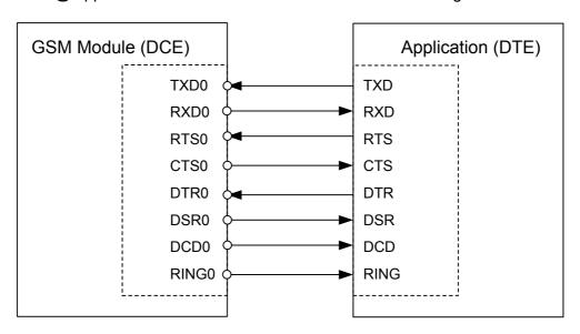
Figure 16: Serial interface ASC0
