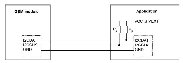
Figure 19: I<sup>2</sup>C interface connected to VCC of application
