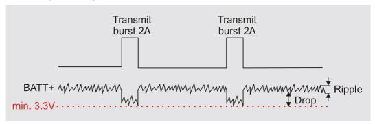
Figure 3: Power supply limits during transmit burst
