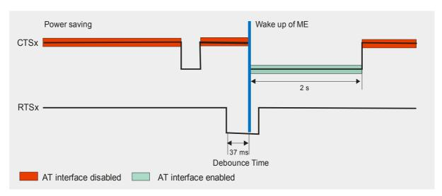
Figure 12: Timing of RTSx signal (if CFUN = 9)
