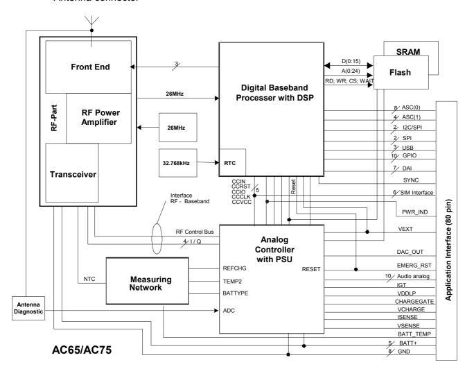
Figure 2: AC65/AC75 block diagram
