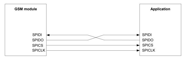
Figure 21: SPI interface
