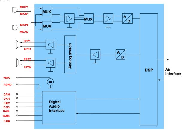
Figure 23: Audio block diagram
