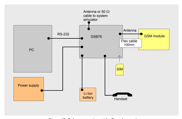
Figure 47: Reference equipment for Type Approval
