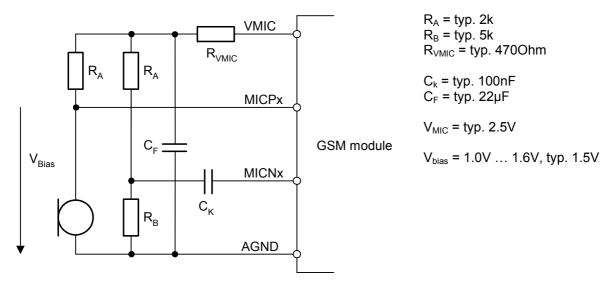
Figure 24: Single ended microphone input
