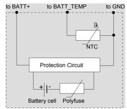
Figure 9: Battery pack circuit diagram
