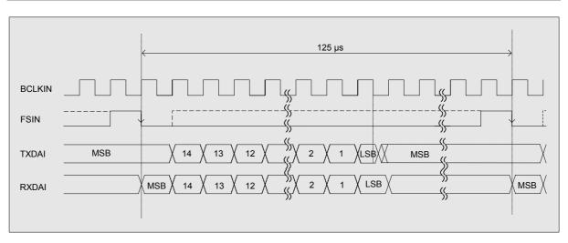
Figure 32: Slave PCM timing, short frame selected
