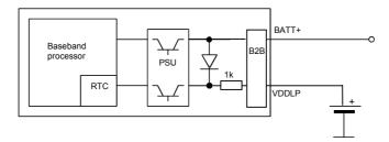
Figure 14: RTC supply from rechargeable battery
