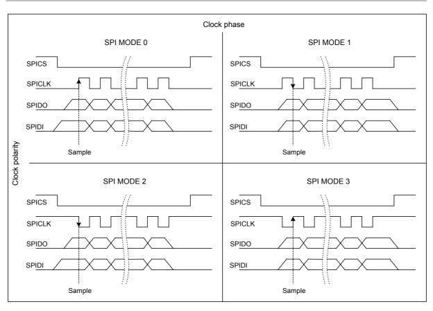
Figure 22: Characteristics of SPI modes
