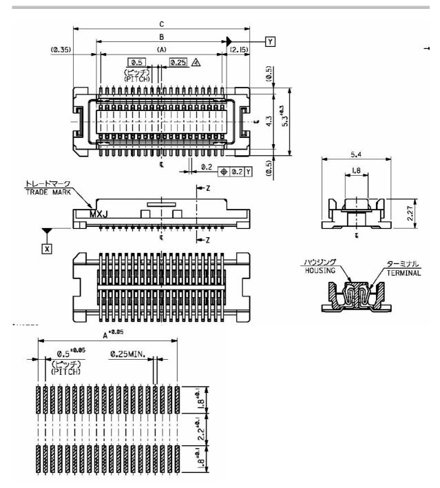
Figure 44: Molex board-to-board connector 52991-0808 on AC65/AC75
