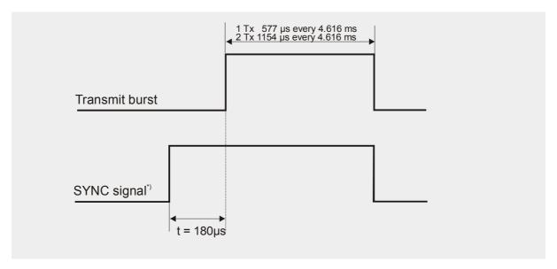
Figure 34: SYNC signal during transmit burst
