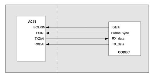
Figure 31: Slave PCM interface application
