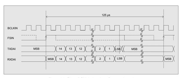
Figure 33: Slave PCM timing, long frame selected
