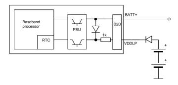
Figure 15: RTC supply from non-chargeable battery
