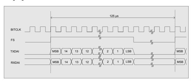
Figure 30: Master PCM timing, long frame selected
