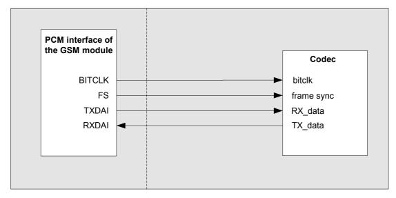
Figure 28: Master PCM interface Application
