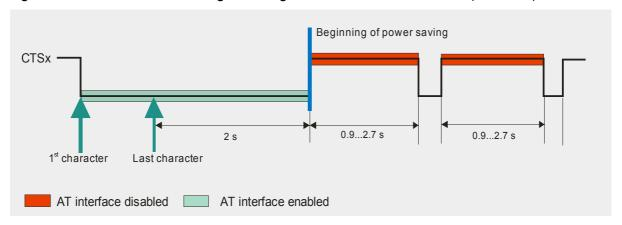
Figure 11: Timing of CTSx signal (if CFUN= 7)
