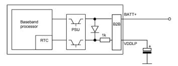
Figure 13: RTC supply from capacitor
