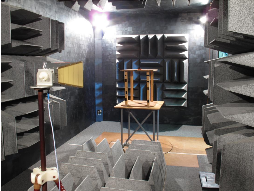
Photograph 2: - MTw sensor, test setup radiated emissions (1 - 18 GHz)
