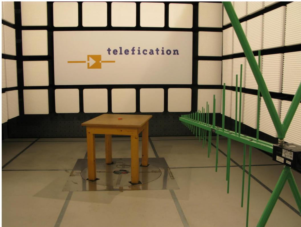
Photograph 1: - MTw sensor, test setup radiated emissions (30 - 1000 MHz)
