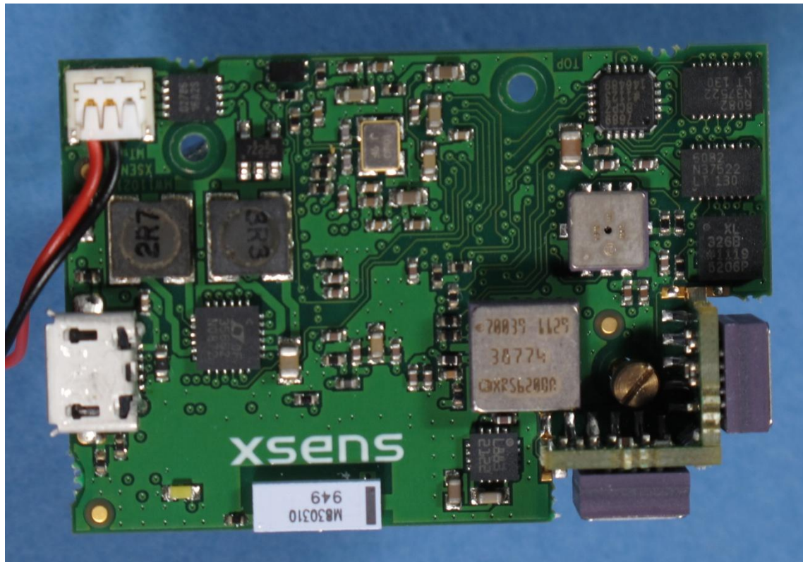
Photograph 3: - MTw sensor, top view of PCB
