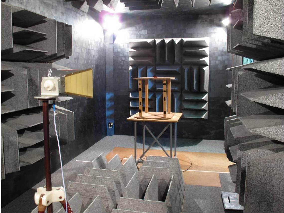
Photograph 2: - MTw , test setup radiated emissions (1 - 18 GHz)
