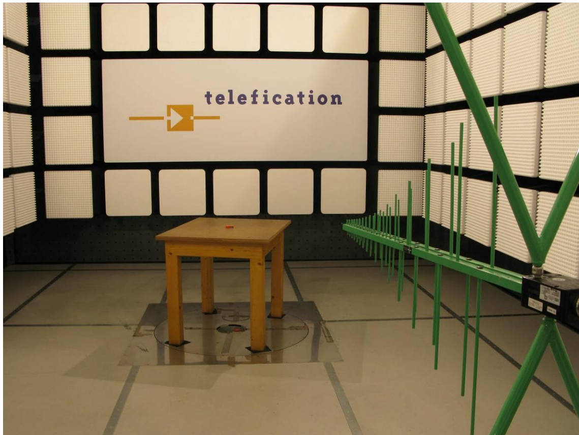
Photograph 1: - MTw , test setup radiated emissions (30 - 1000 MHz)
