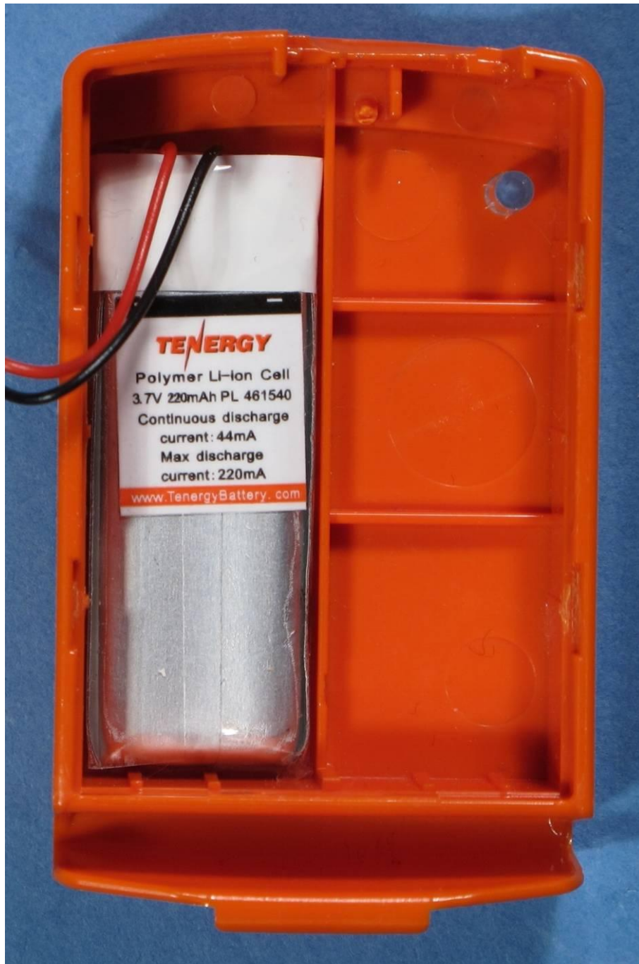
Photograph 2: - MTw sensor, battery view
