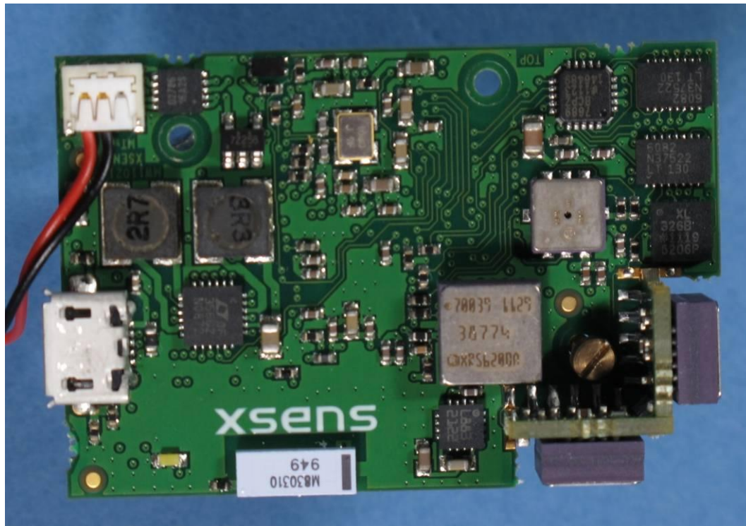
Photograph 3: - MTw sensor, top view of PCB
