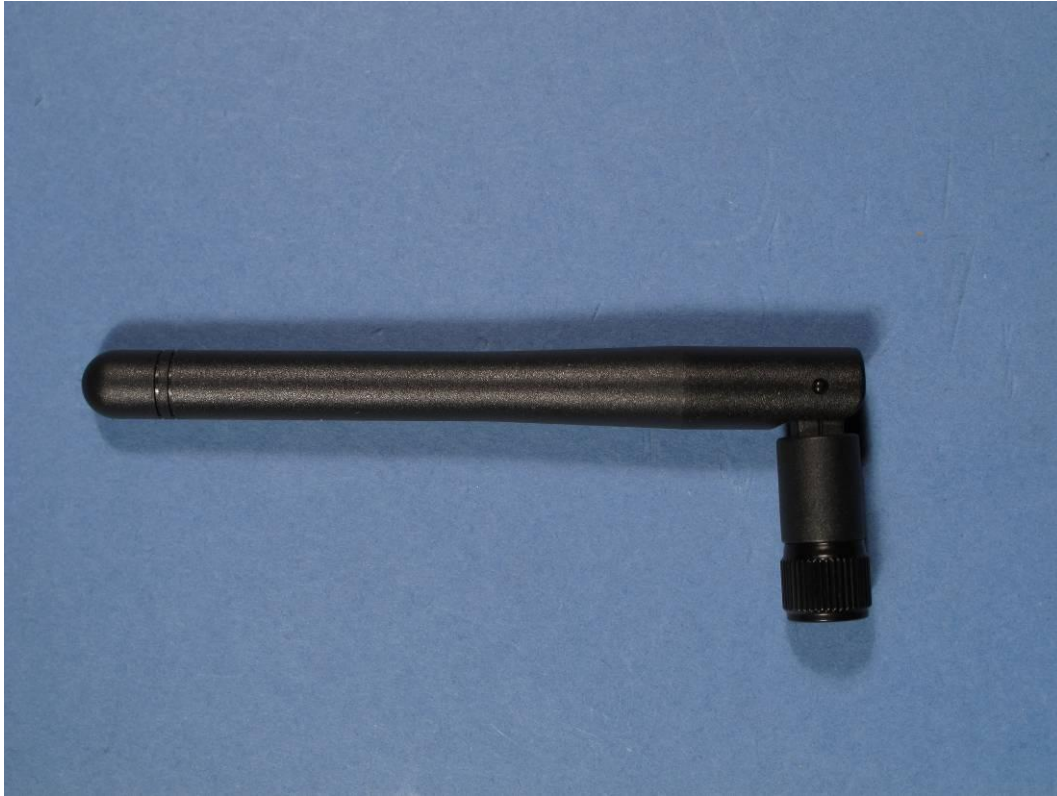
Photograph 4: - AW-A Wireless base station, antenna
