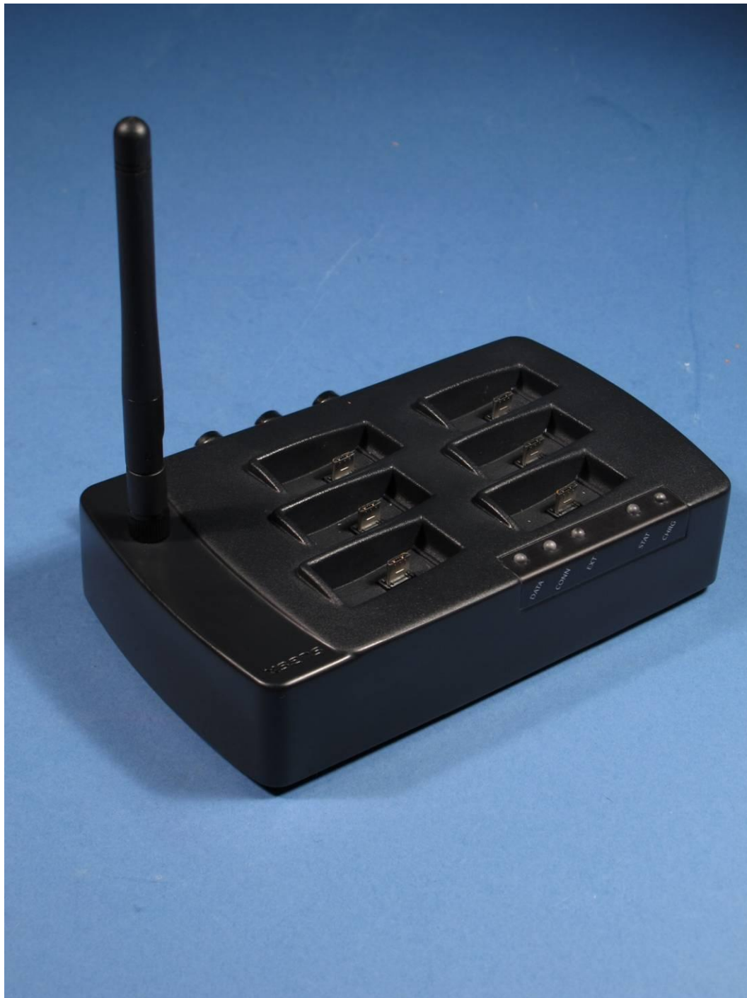
Photograph 1: - AW-A Wireless base station, front view
