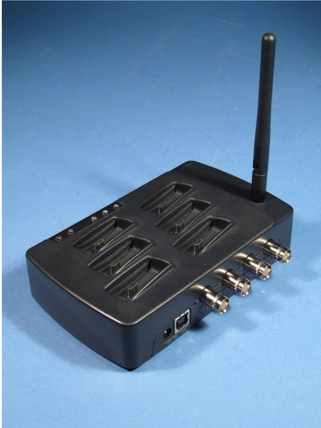
Photograph 2: - AW-A Wireless base station, rear view
