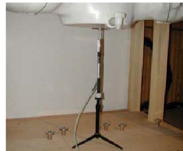
Figure 9.1 Dipole Verification Test Setup Diagram & Photo
