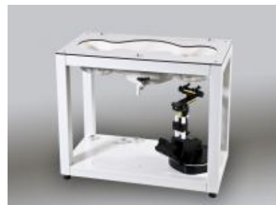
Figure 3.6 SAM Twin Phantom
