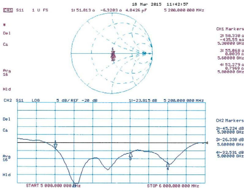
**Impedance Measurement Plot for Head TSL (5250, 5500, 5750)**
