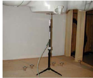
Figure 9.1 Dipole Verification Test Setup Diagram & Photo
