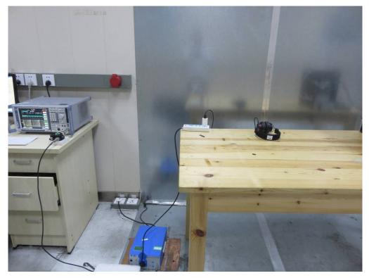
FCC RADIATED EMISSION TEST SETUP
