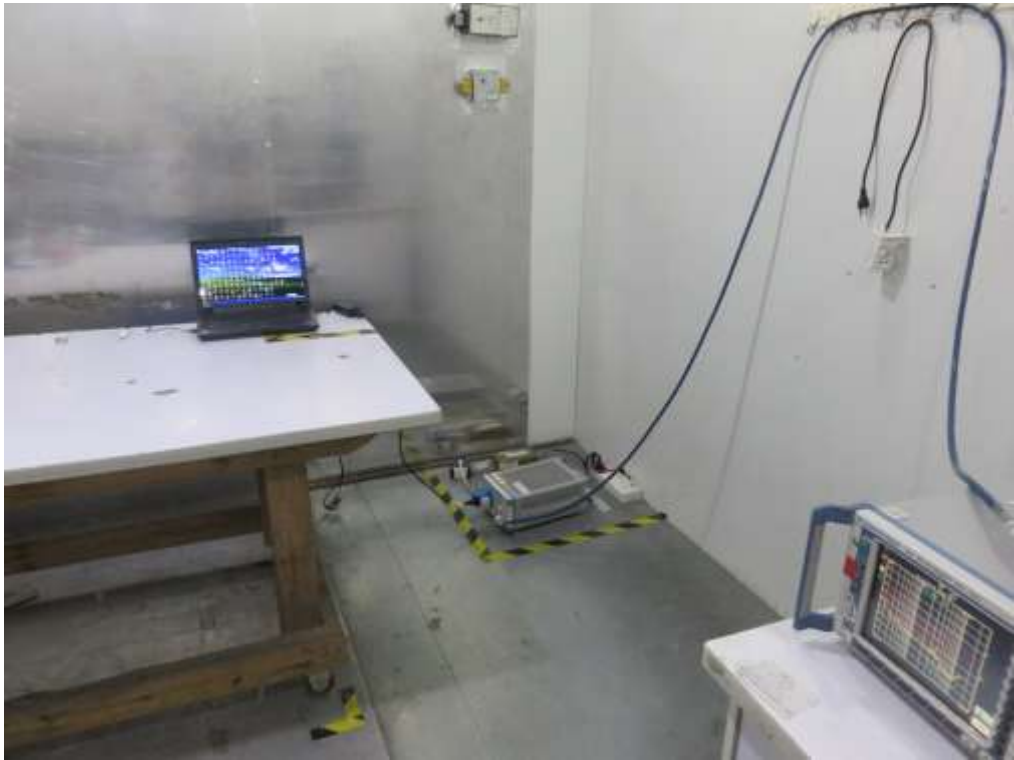
FCC RADIATED EMISSION TEST SETUP
