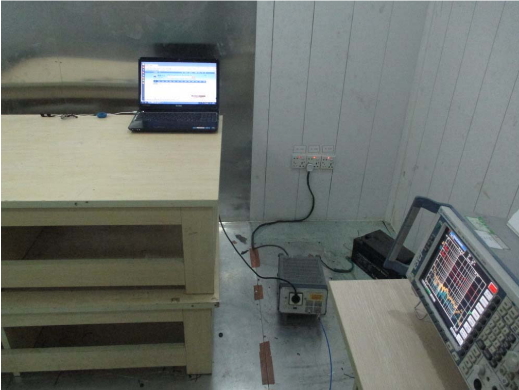
FCC RADIATED EMISSION TEST SETUP
