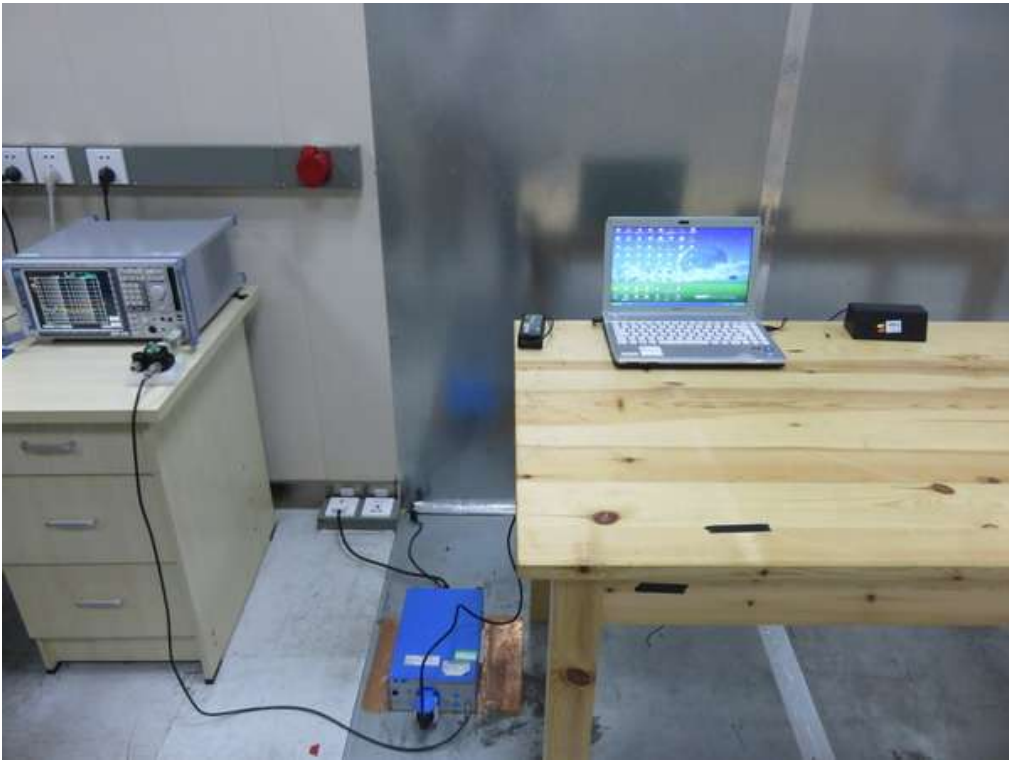
FCC RADIATED EMISSION TEST SETUP
