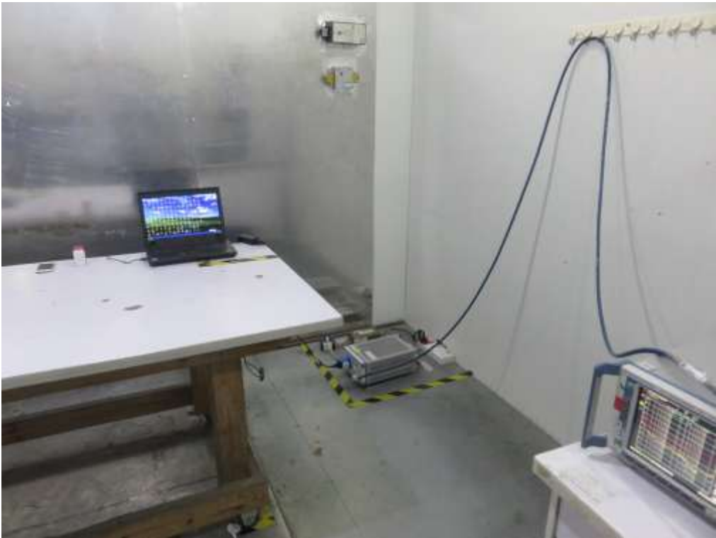
FCC RADIATED EMISSION TEST SETUP
