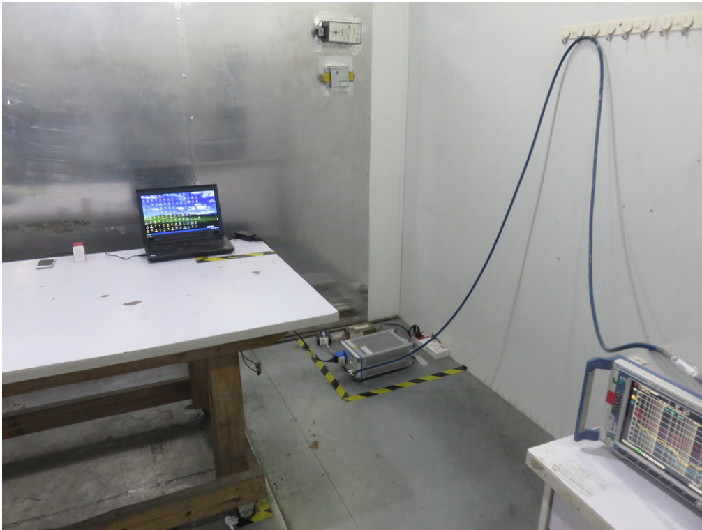
FCC RADIATED EMISSION TEST SETUP
