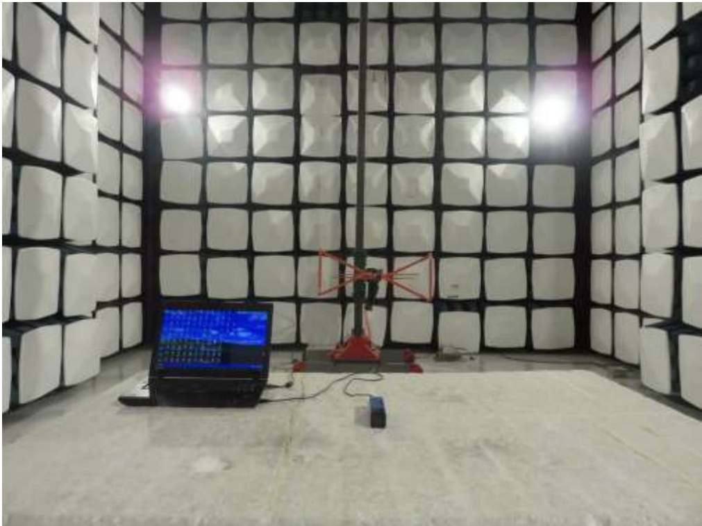
FCC RADIATED EMISSION TEST SETUP
