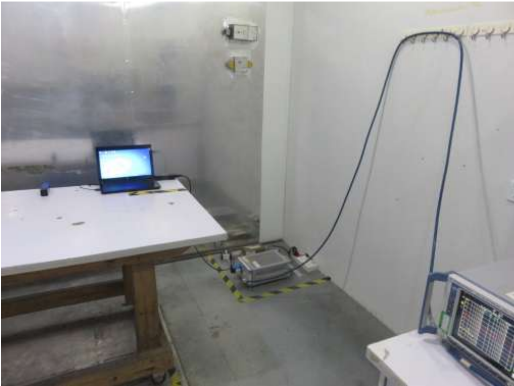
FCC RADIATED EMISSION TEST SETUP
