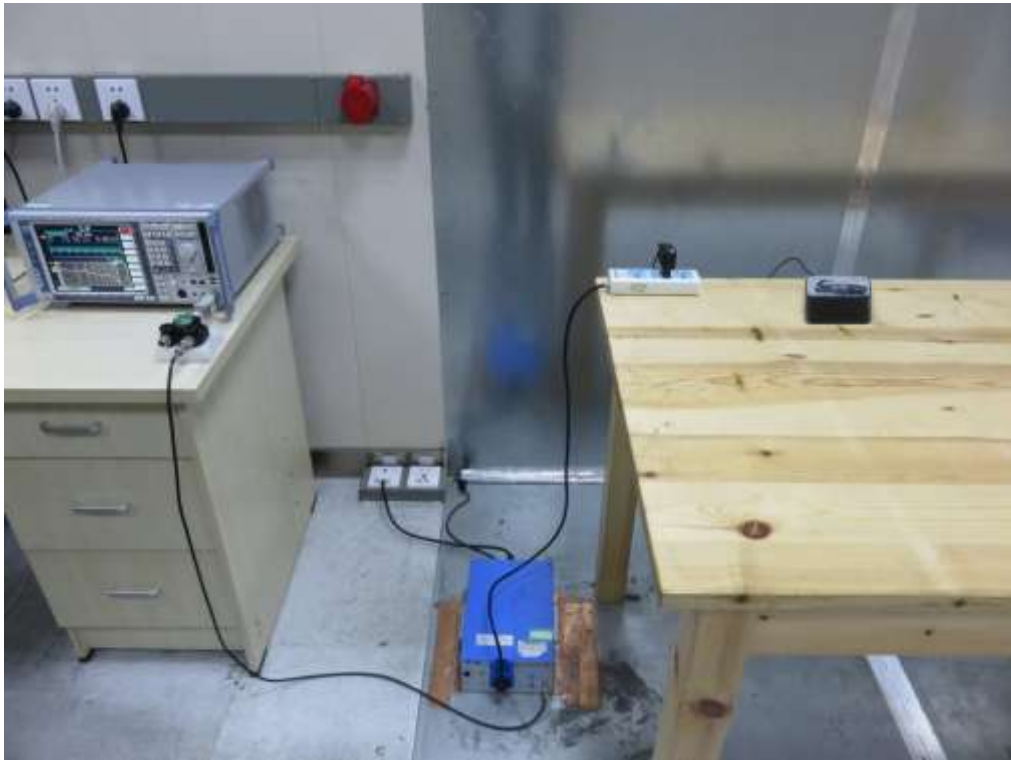
FCC RADIATED EMISSION TEST SETUP
