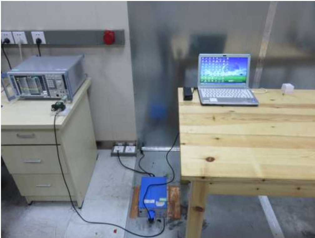
FCC RADIATED EMISSION TEST SETUP
