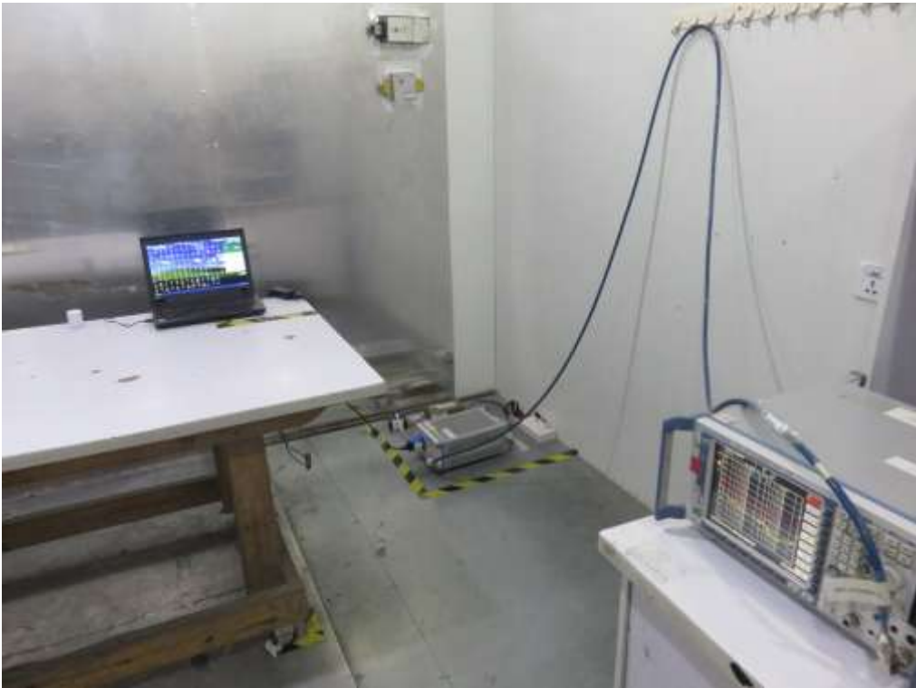
FCC RADIATED EMISSION TEST SETUP
