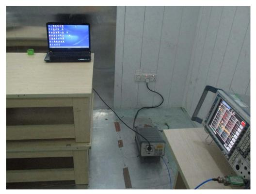
FCC RADIATED EMISSION TEST SETUP
