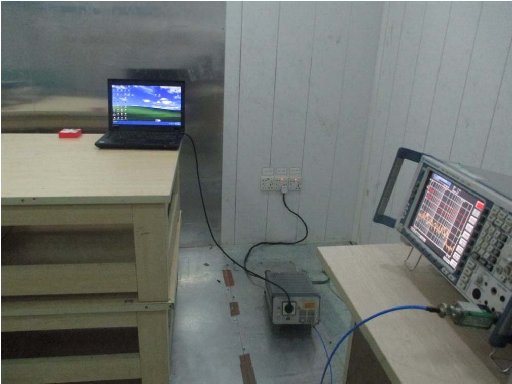
FCC RADIATED EMISSION TEST SETUP
