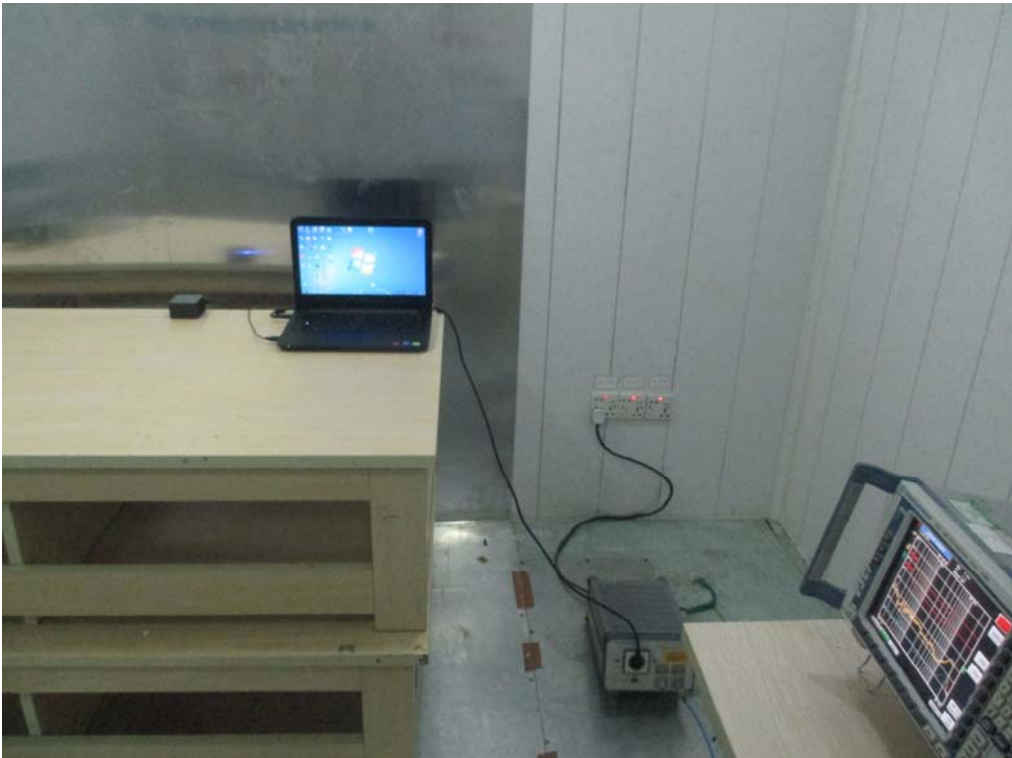
FCC RADIATED EMISSION TEST SETUP
