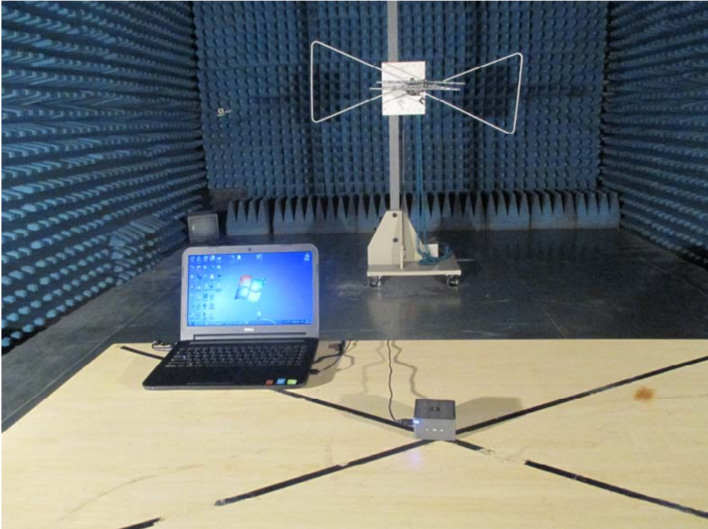
FCC RADIATED EMISSION TEST SETUP
