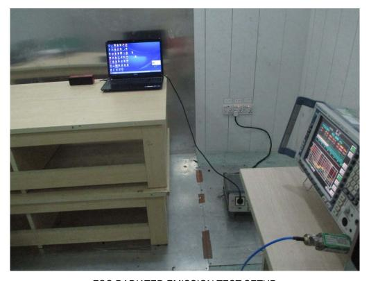
FCC RADIATED EMISSION TEST SETUP
