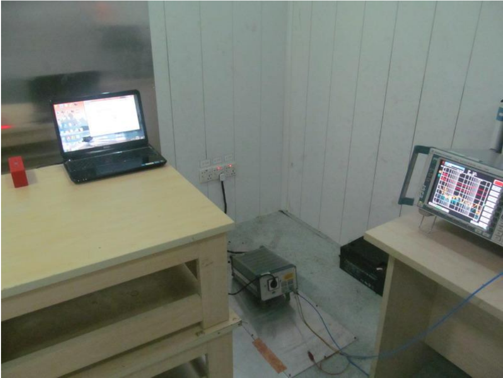
FCC RADIATED EMISSION TEST SETUP
