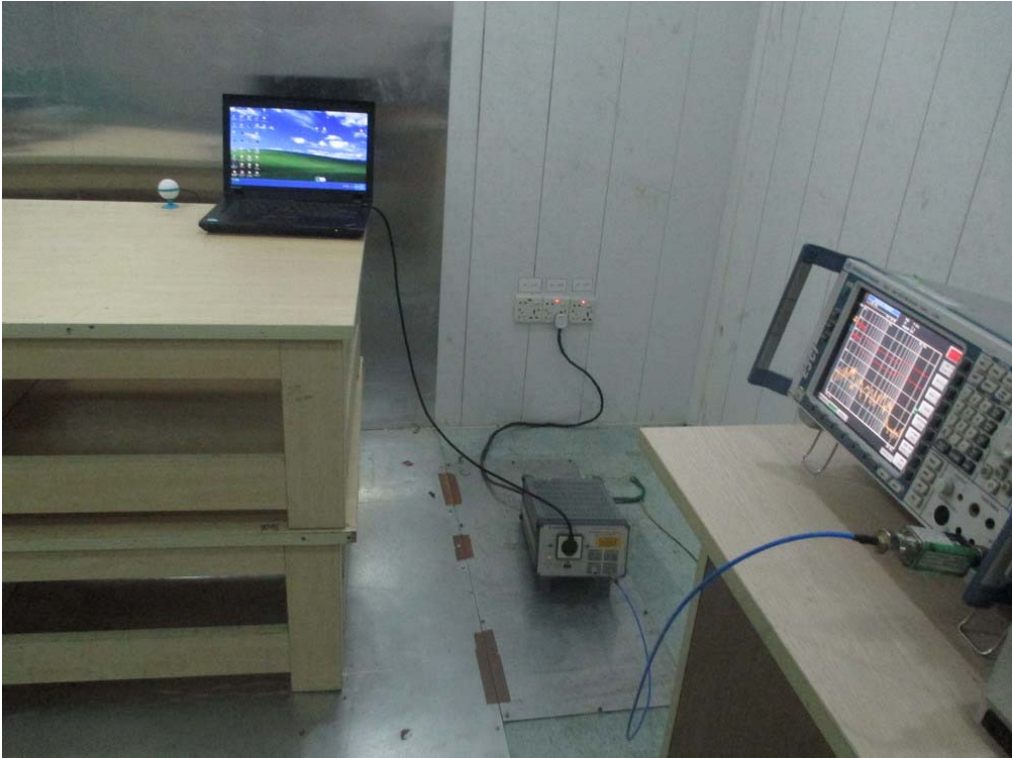
FCC RADIATED EMISSION TEST SETUP
