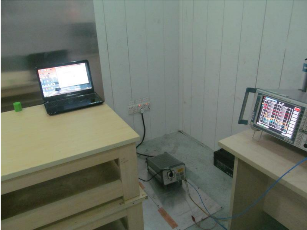
FCC RADIATED EMISSION TEST SETUP
