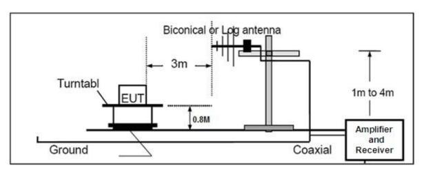
RADIATED EMISSION TEST SETUP ABOVE 1000MHz
