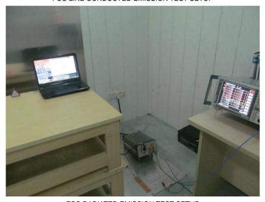
FCC RADIATED EMISSION TEST SETUP
