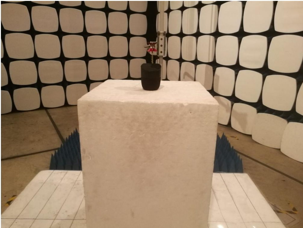
RADIATED EMISSION TEST SETUP ABOVE 1GHZ
