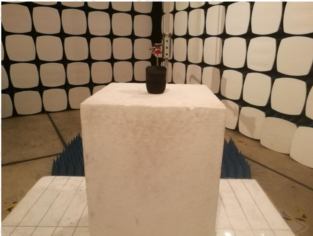
RADIATED EMISSION TEST SETUP ABOVE 1GHZ
