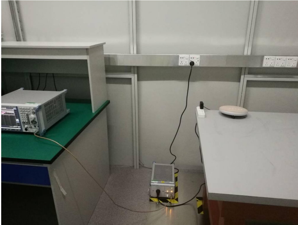
FCC RADIATED EMISSION TEST SETUP
