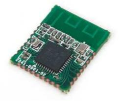
BT0001 build-in 8051 MCU, in-system software stack programmable flash memory, 8-KB RAM, and many multiple configuration options other powerful supporting features and peripherals, including UART, IIC and GPIO. BT0001 is 25-pin I/O interface (with back size 9 pin) to bring UART, I<sup>2</sup>C or GPIO data to wireless through Bluetooth BLE protocol. BT0001 build-in the hi-efficiency PCB antenna for compact and easy assembly application.
