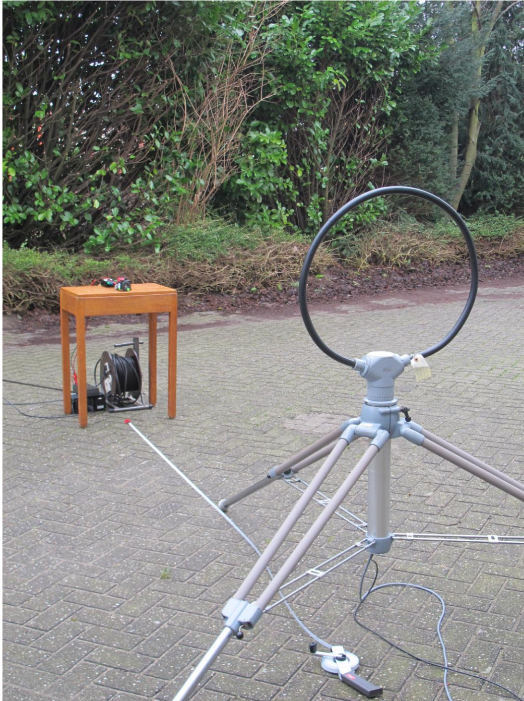
Photograph 1: Test setup radiated emissions < 30 MHz
