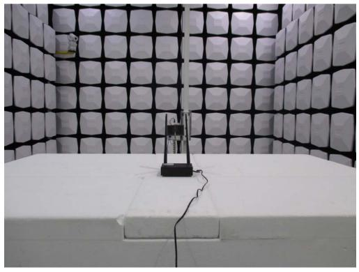
Test Mode: Mode 4: WCDMA Band 2\_Idle Mode Description: Back View of Radiated Spurious Emission Test Setup (Horn)
