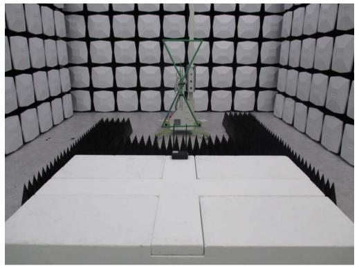
Test Mode: Mode 1: WCDMA Band 5\_Link Mode Description: Back View of Radiated Spurious Emission Test Setup
