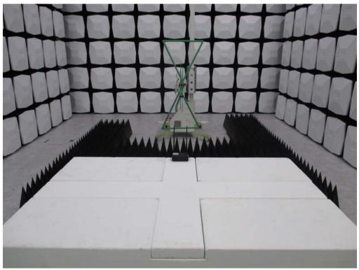
Test Mode: Mode 2: WCDMA Band 5\_Idle Mode Description: Back View of Radiated Spurious Emission Test Setup
