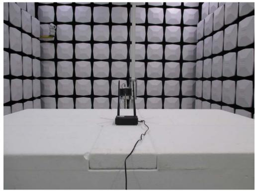
Test Mode: Mode 1: WCDMA Band 5\_Link Mode Description: Back View of Radiated Spurious Emission Test Setup (Horn)
