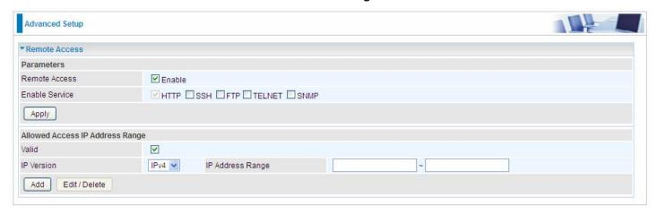
**Remote Access:** Select "Enable" to allow management access from remote side (mostly from internet). If disabled, no remote access is allowed for any IPs even if you set allowed access IP address. So, please note that enabling remote access is an essential step before granting remote access to IPs.
