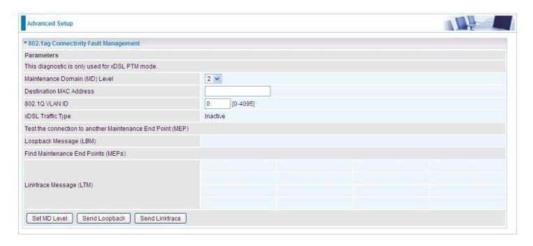
**Maintenance Domain (MD) Level:** Maintenance Domains (MDs) are management spaces on a network, typically owned and operated by a single entity. MDs are configured with Names and Levels, where the eight levels range from 0 to 7. A hierarchal relationship exists between domains based on levels. The larger the domain, the higher the level value.
