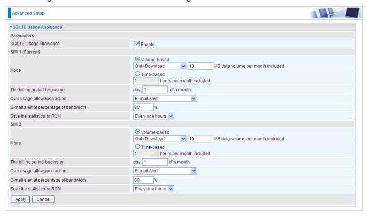
**3G/LTE Usage Allowance:** Enable to monitor 3G/LTE usage.
