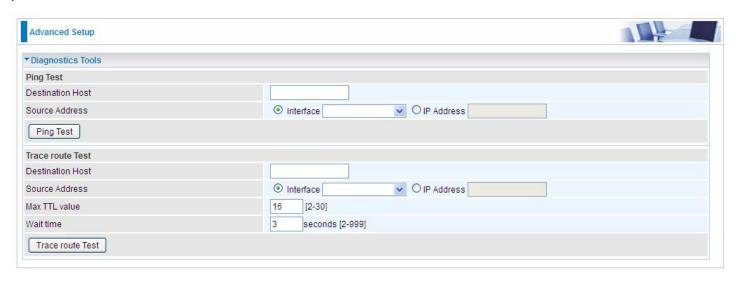
**Ping Test:** to verify the connectivity between source and destination.
