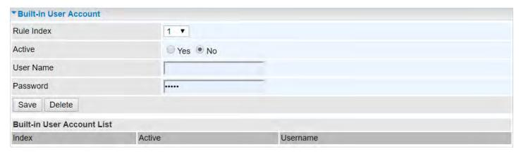
Rule Index: The numeric rule indicator. The maximum entry is up to 16.
