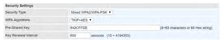
**WPA Algorithms:** TKIP (Temporal Key Integrity Protocol) or AES (Advanced Encryption System) utilizes a stronger encryption method and incorporates Message Integrity Code (MIC) to provide protection against hackers.
