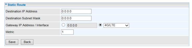
**Destination IP Address:** This is the destination subnet IP address.
