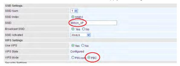
2. Launch the wireless client's WPS Utility (e.g. Ralink Utility). Set the Config Mode as **Enrollee**. Then press the **WPS button** and choose the correct AP (e.g. **Billion\_AP**) from the WPS AP List section before pressing the **PBC** button to run the scan.
