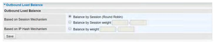
User can distribute outbound traffic based on Session Mechanism or IP Hash Mechanism.
