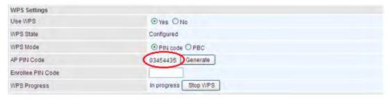
2. Launch the wireless client's WPS utility (e.g. Ralink Utility). Set the Config Mode as Registrar. Enter the PIN number in the PIN Code (e.g. 03454435) column then choose the correct AP (e.g. Billion\_AP) from the WPS AP List before pressing the PIN button to run the scan.
