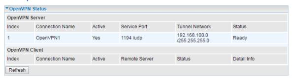
Index #: The numeric OpenVPN tunnel/ rule.
