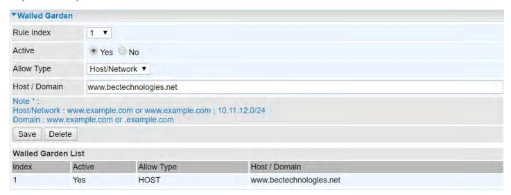
Rule Index: The numeric rule indicator. The maximum entry is up to 16.
