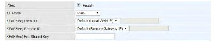
**IKE Mode:** IKE, Internet Key Exchange, is the mechanism to negotiate and exchange parameters and keys between IPSec peers to establish security associations (SA). Select Main or Aggressive mode.
