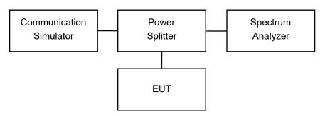
Radiated Spurious Measurement: below 1GHz
