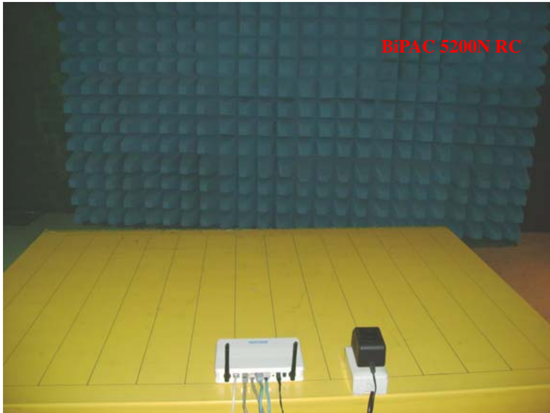
Photo 2: Radiated Emission Test set-up photo
