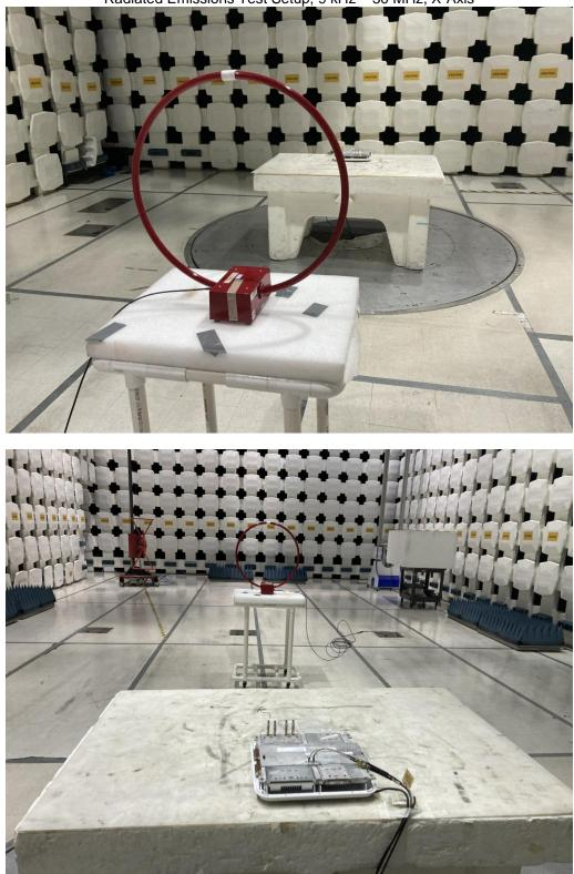
Radiated Emissions Test Setup, 9 kHz - 30 MHz, X-Axis
