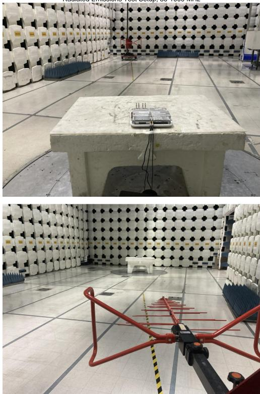
Radiated Emissions Test Setup, 30-1000 MHz
