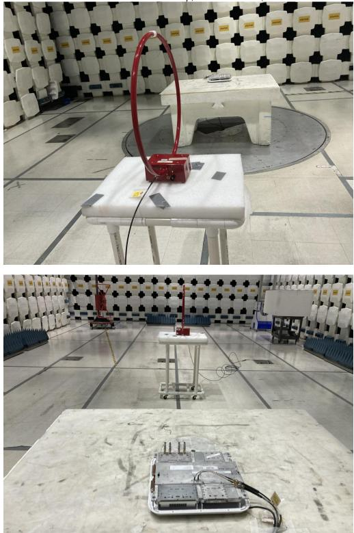
Radiated Emissions Test Setup, 9 kHz – 30 MHz, Y-Axis
