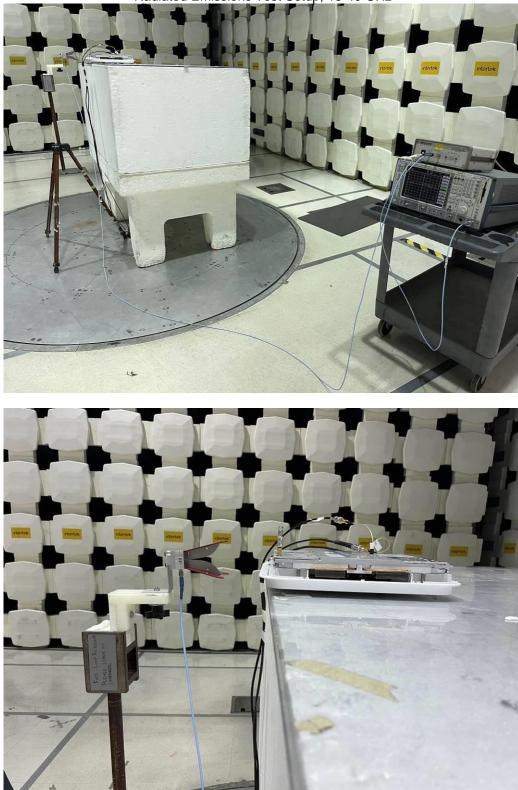
Radiated Emissions Test Setup, 18-40 GHz
