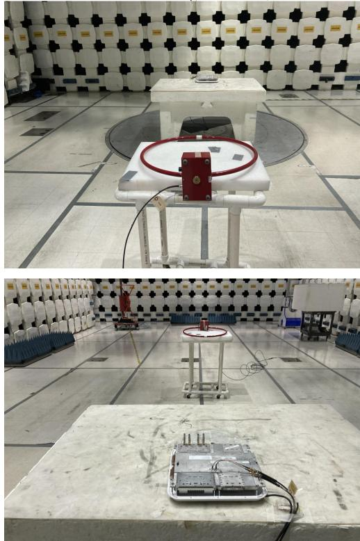
Radiated Emissions Test Setup, 9 kHz - 30 MHz, Z-Axis
