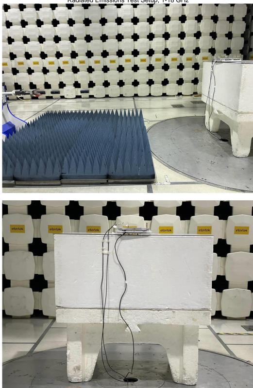
Radiated Emissions Test Setup, 1-18 GHz
