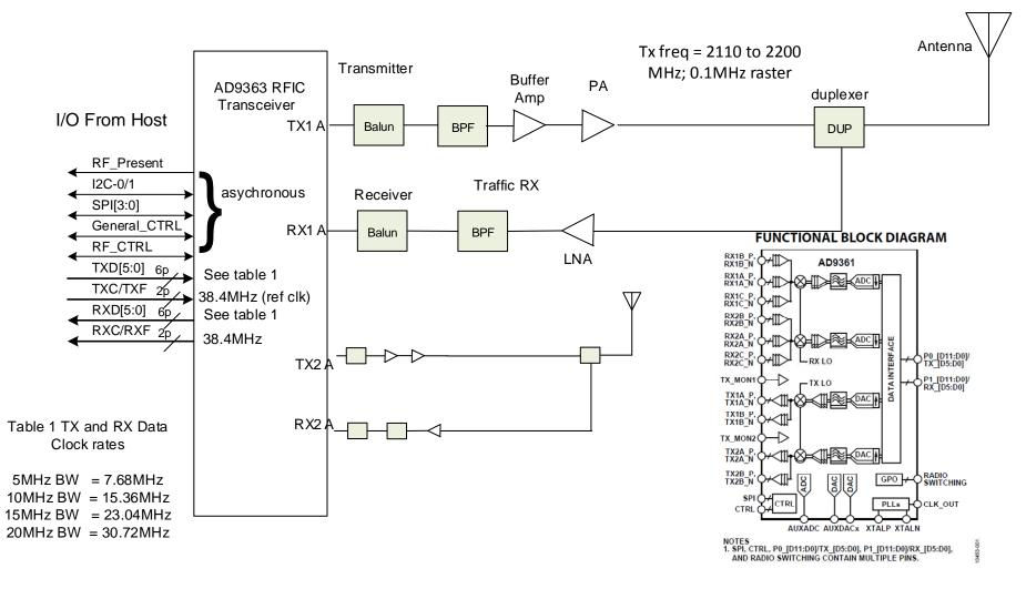
Figure 1b below shows a typical radio module block diagram.
