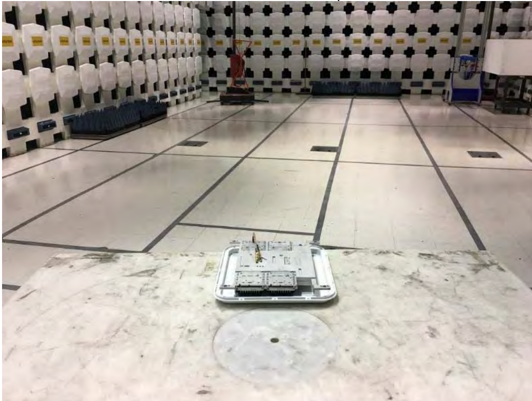
30-1000 MHz Test Setup
