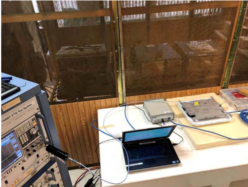
Antenna Port Conducted Test Setup
