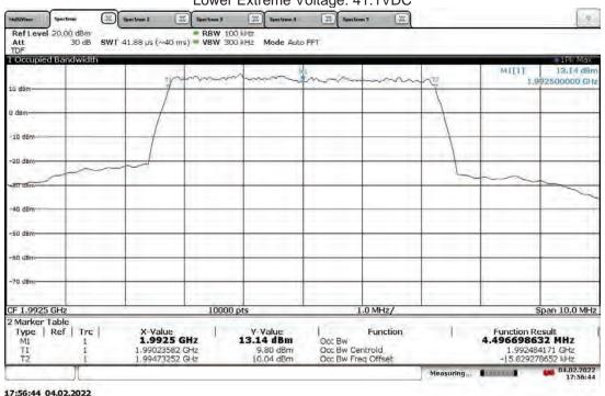
Slot 0 (Band 25), ANT1, Modulation: QPSK, Bandwidth: 5 MHz, Low Channel 1932.5 MHz, (4G LTE)
