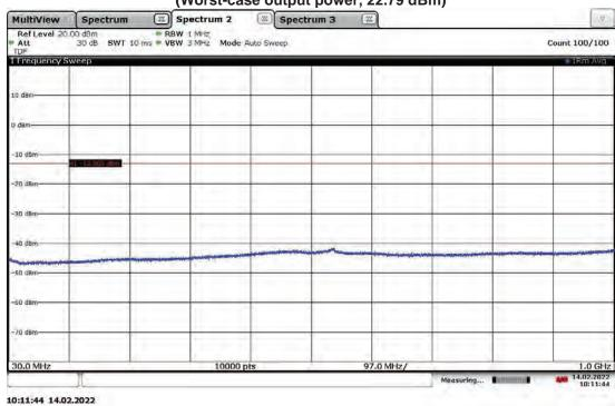
Antenna Port (ANT1) Conducted Emissions, 1-20 GHz Band 25(4G LTE), Mid Channel 1962.5 MHz, BW 15 MHz, Modulation QPSK (Worst-case output power, 22.79 dBm)
