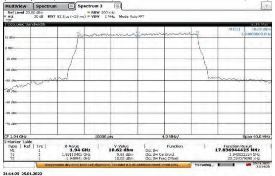
Slot 0 (Band 25), ANT1, Modulation: QPSK, Bandwidth: 20 MHz Low Channel 1940 MHz, 50 °C (5G nR)
