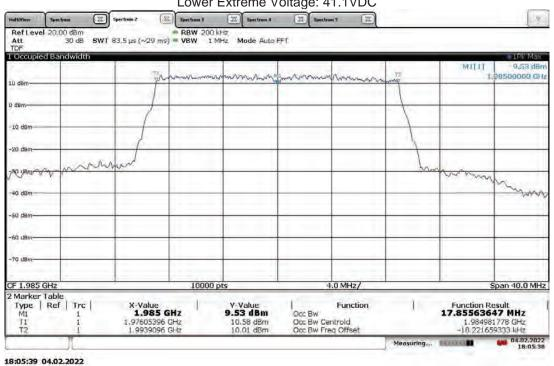
Slot 0 (Band 25), ANT1, Modulation: QPSK, Bandwidth: 20 MHz, Low Channel 1940 MHz (5G nR) Nominal Voltage: 48 VDC
