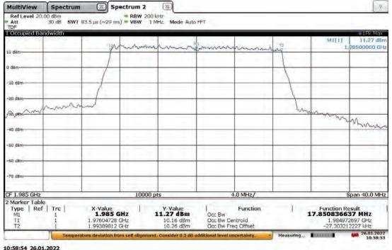
Slot 0 (Band 25), ANT1, Modulation: QPSK, Bandwidth: 20 MHz High Channel 1985 MHz, 50 °C (5G nR)
