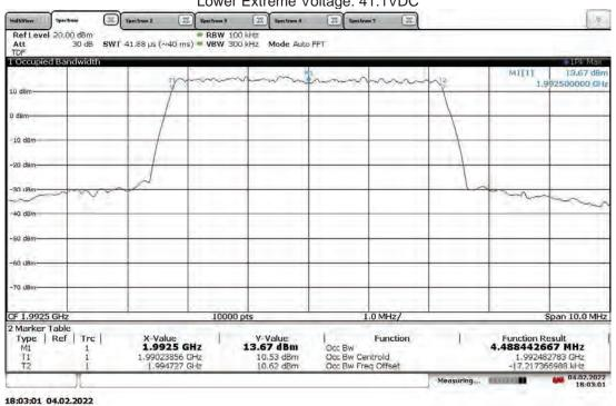
Slot 0 (Band 25ANT1, Modulation: QPSK, Bandwidth: 5 MHz, Low Channel 1932.5 MHz (5G nR) Nominal Voltage: 48 VDC
