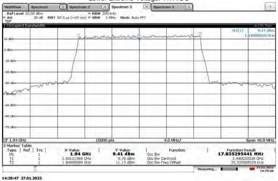
Slot 0 (Band 25), ANT1, Modulation: QPSK, Bandwidth: 20 MHz, High Channel 1985 MHz (4G LTE) Lower Extreme Voltage: 41.1VDC
