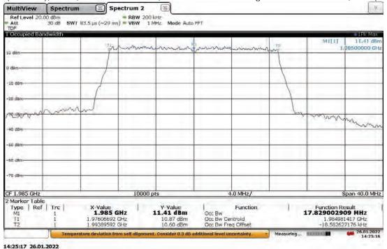
Slot 0 (Band 25), ANT1, Modulation: QPSK, Bandwidth: 20 MHz High Channel 1985 MHz, -10 °C (5G nR)
