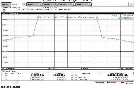
Slot 0 (Band 25), ANT1, Modulation: QPSK, Bandwidth: 20 MHz, Low Channel 1940 MHz (5G nR)
