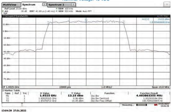
Slot 0 (Band 25), ANT1, Modulation: QPSK, Bandwidth: 5 MHz, High Channel 1992.5 MHz (4G LTE)
