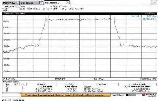
Slot 0 (Band 25), ANT1, Modulation: QPSK, Bandwidth: 20 MHz Low Channel 1940 MHz, -30 °C (5G nR)
