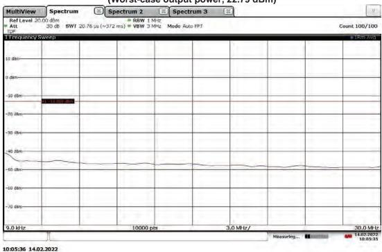
Antenna Port (ANT0) Conducted Emissions, 30 MHz-1000 MHz Band 25(4G LTE), Mid Channel 1962.5 MHz, BW 15 MHz, Modulation QPSK (Worst-case output power, 22.79 dBm)
