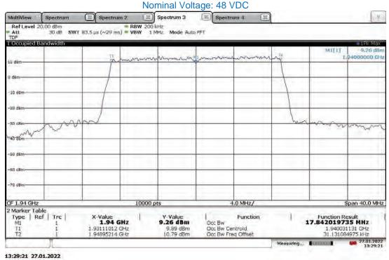
Slot 0 (Band 25), ANT1, Modulation: QPSK, Bandwidth: 20 MHz, High Channel 1980 MHz (4G LTE)
