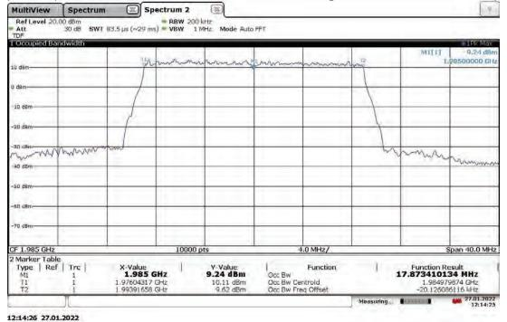
Slot 0 (Band 25), ANT1, Modulation: QPSK, Bandwidth: 20 MHz High Channel 1985 MHz, -20 °C (5G nR)
