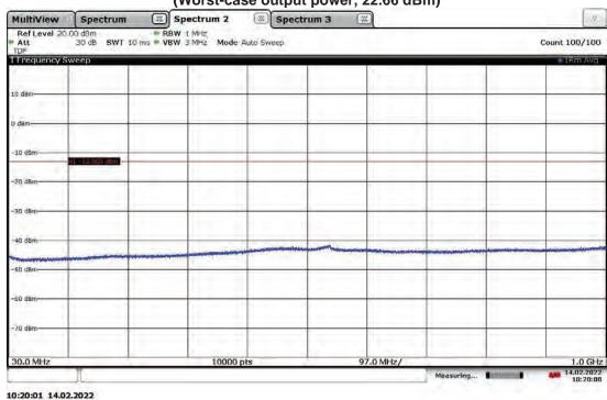
Antenna Port (ANT1) Conducted Emissions, 1-20 GHz Band 25(4G LTE), High Channel 1985 MHz, BW 20 MHz, Modulation 64QAM (Worst-case output power, 22.66 dBm)
