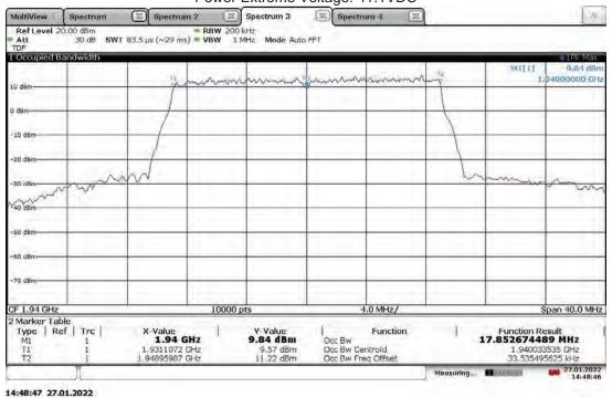
Slot 0 (Band 25), ANT1, Modulation: QPSK, Bandwidth: 20 MHz, High Channel1985 MHz (5G nR) Lower Extreme Voltage: 41.1VDC
