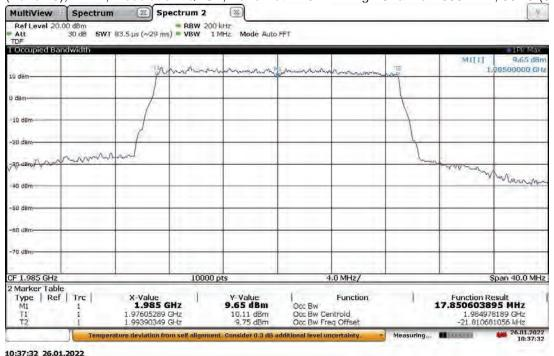
Slot 0 (Band 25), ANT1, Modulation: QPSK, Bandwidth: 5 MHz, Low Channel 1932.5 MHz, (4G LTE) Lower Extreme Voltage: 41.1VDC
