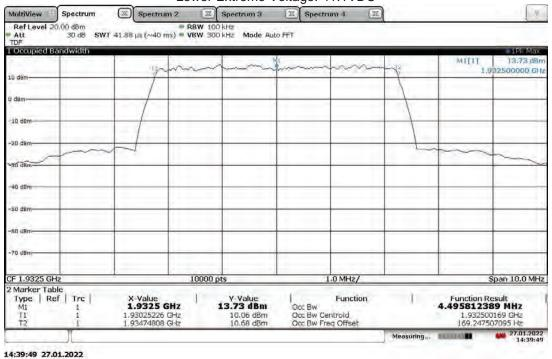
Slot 0 (Band 25), ANT1, Modulation: QPSK, Bandwidth: 5 MHz, High Channel 1992.5 MHz (5G nR) Lower Extreme Voltage: 41.1VDC
