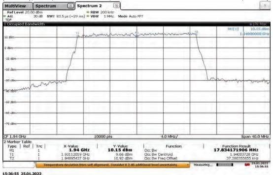
Slot 0 (Band 25), ANT1, Modulation: QPSK, Bandwidth: 20 MHz Low Channel 1940 MHz, -20 °C (5G nR)
