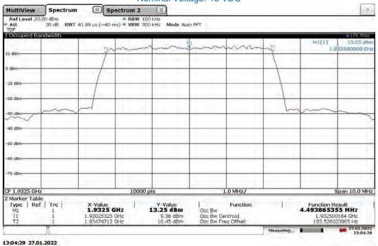
Slot 0 (Band 25), ANT1, Modulation: QPSK, Bandwidth: 5 MHz, High Channel 1992.5 MHz (5G nR) Nominal Voltage: 48 VDC
