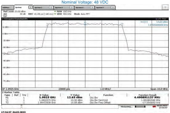
Slot 0 (Band 25), ANT1, Modulation: QPSK, Bandwidth: 5 MHz, Low Channel 1932.5 MHz (4G LTE) Upper Extreme Voltage: 57.0VDC
