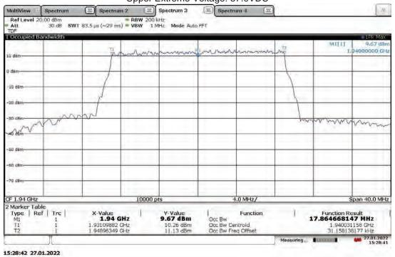
Slot 0 (Band 25), ANT1, Modulation: QPSK, Bandwidth: 20 MHz, High Channel 1985 MHz (5G nR) Upper Extreme Voltage: 57.0VDC
