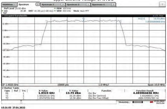
Slot 0 (Band 25), ANT1, Modulation: QPSK, Bandwidth: 5 MHz, High Channel 1992.5 MHz (5G nR) Upper Extreme Voltage: 57.0VDC
