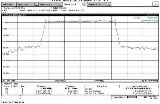
Slot 0 (Band 25), ANT1, Modulation: QPSK, Bandwidth: 20 MHz, High 1985 MHz (4G LTE)
