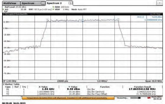
Slot 0 (Band 25), ANT1, Modulation: QPSK, Bandwidth: 20 MHz High Channel 1985 MHz, 0 °C (5G nR)
