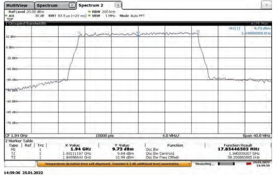
Slot 0 (Band 25), ANT1, Modulation: QPSK, Bandwidth: 20 MHz Low Channel 1940 MHz, -10 °C (5G nR)
