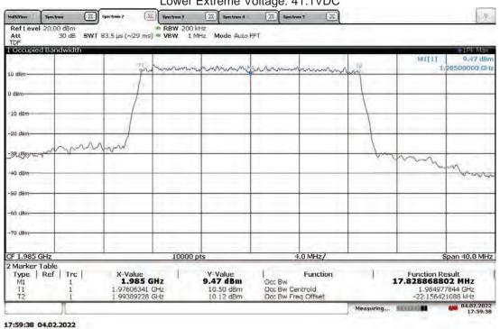
Slot 0 (Band 25), ANT1, Modulation: QPSK, Bandwidth: 20 MHz, Low Channel 1940 MHz (4G LTE)
