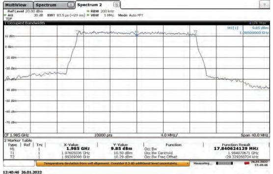
Slot 0 (Band 25), ANT1, Modulation: QPSK, Bandwidth: 20 MHz High Channel 1985 MHz, 30 °C (5G nR)
