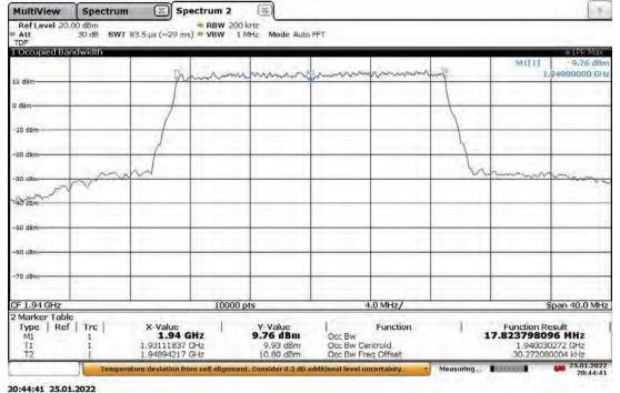
Slot 0 (Band 25), ANT1, Modulation: QPSK, Bandwidth: 20 MHz Low Channel 1940 MHz, 40 °C (5G nR)
