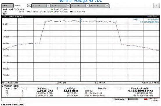
Slot 0 (Band 25), ANT1, Modulation: QPSK, Bandwidth: 5 MHz, Low Channel 1932.5 MHz (5G nR)
